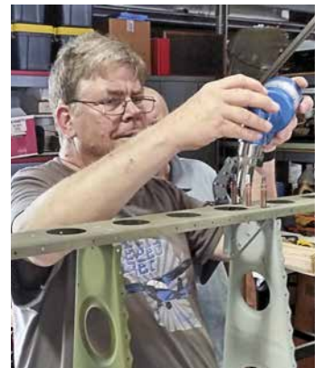
This shows me working on riveting part of the fuselage.
