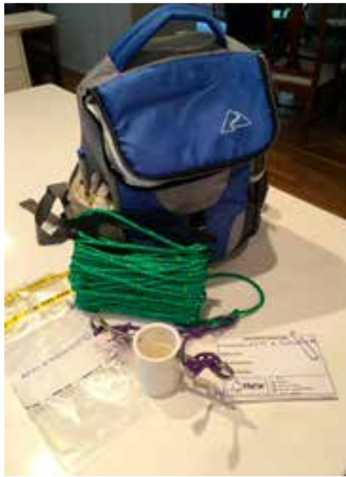
This is a water-testing kit. Riverkeeper trains the volunteers so they know the correct way to collect creek water without contaminating the samples. Riverkeeper also provides each volunteer with a kit that contains the necessary materials to collect and store samples.
